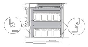
While holding the strap 1, pull the DIMM adapter toward the front 2 to remove it.
